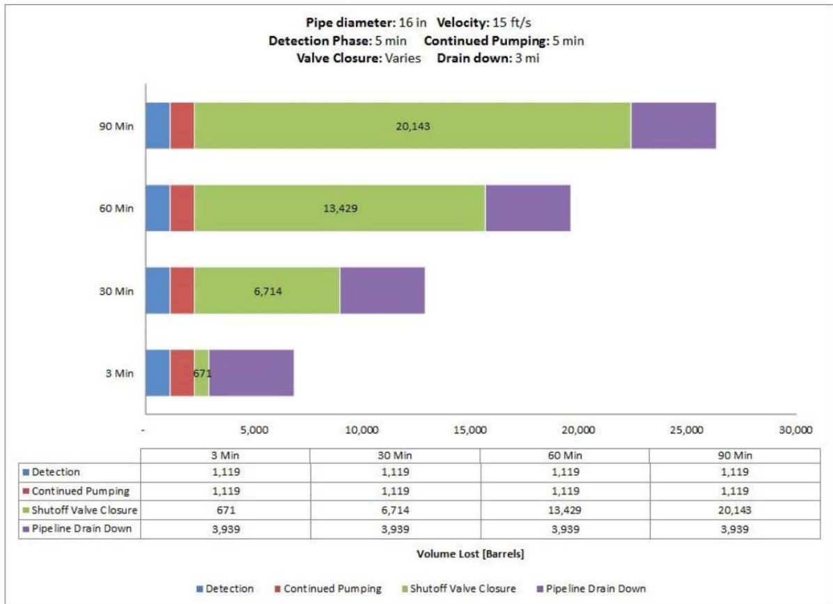
FIGURE 5. Leakage from a pipeline carrying liquid propane following leak detection. This pipeline is of 16-inch diameter, at 1,480 psi pressure providing liquid movement at 15 feet per second, with 100 feet local elevation change within 3 miles of the shutoff valve (Oland et al. 2012).
